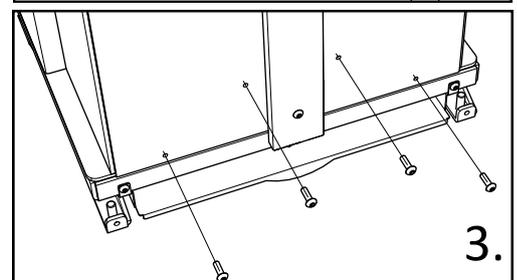
4. Attach the rear outside airbox with the 4 x screws provided. NEVER leave any of the holes empty as they may create an air leak into the stove.
